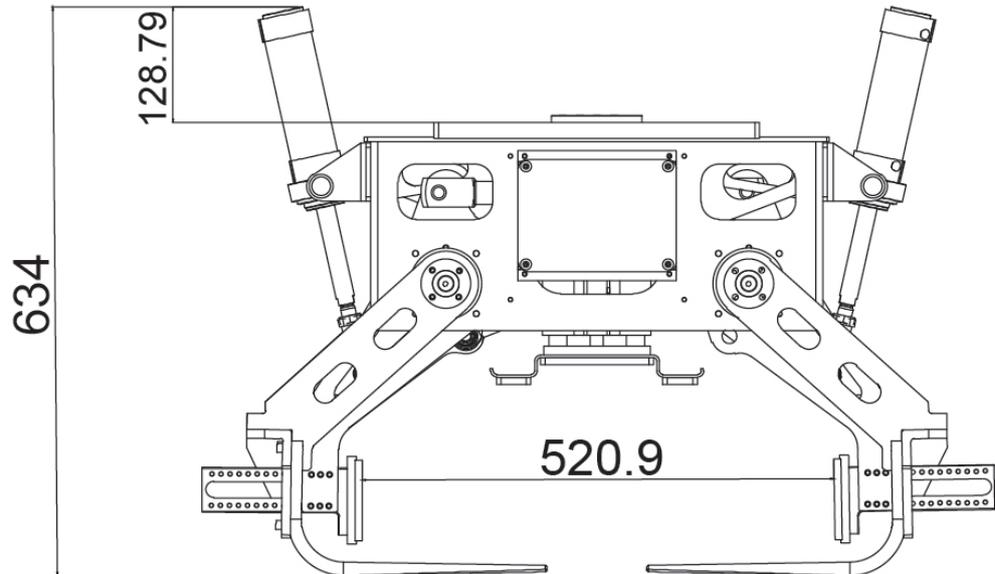
Size with claws in minimum working position and push plates in minimum working position
