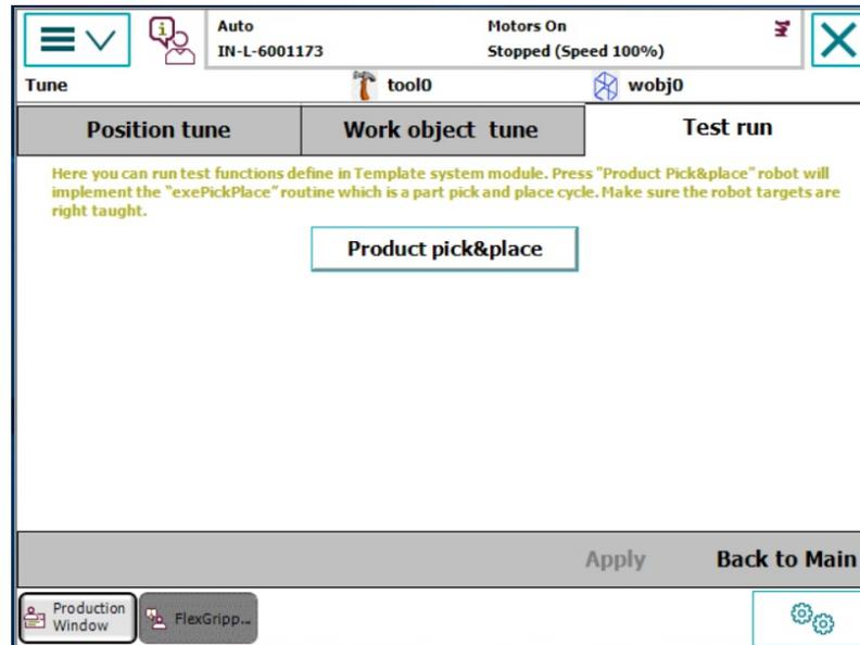
Press the Product Pick&place button, the robot implements the exePickPlace routing which includes a part pick and place cycle.
