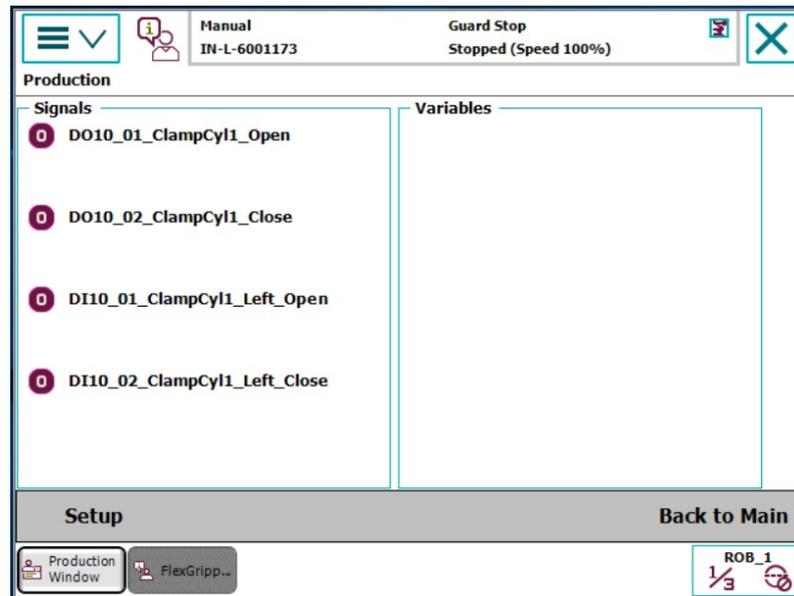
Touch the Setup button, the interface with signal list shows.
