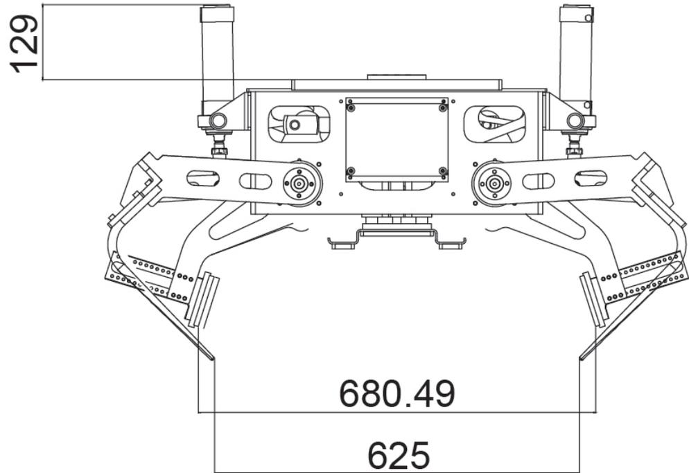
Size with claws in maximum working position and push plates in minimum working position
