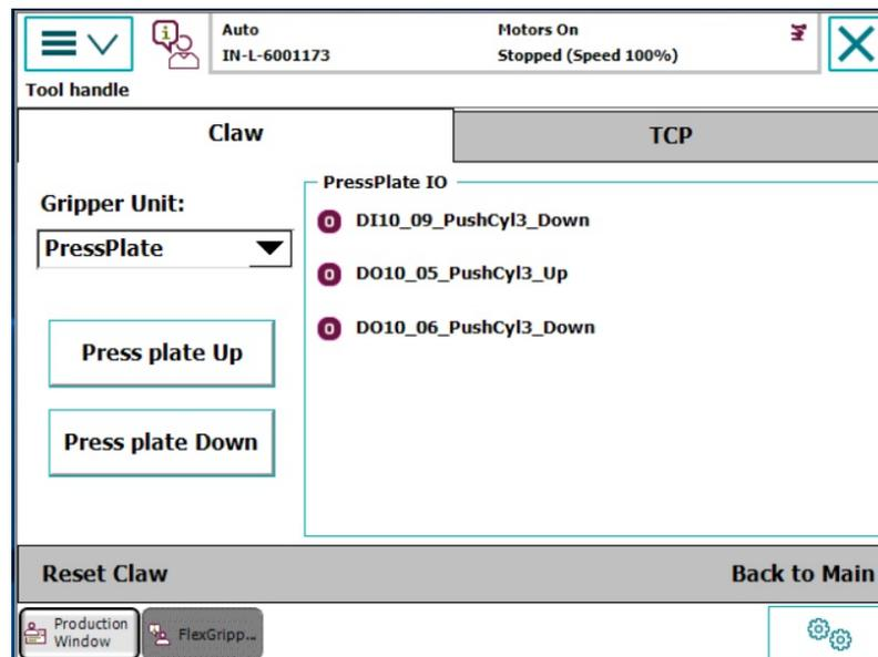
You can operate the functions displayed and check if the corresponding signals status is correct. The functions displayed are Claw open, Claw close, Press plate up and Press plate down.
